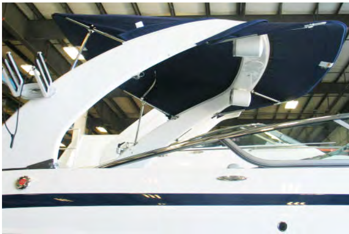
TYPICAL POWER TOWER- SUNSHADES IN CRUISE POSITION
